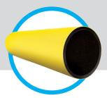
PE80 Yellow Pipe is used for pressurised gas supply. Pipes up to 63mm in diameter are solid yellow PE80; from 75 to 225mm in diameter, pipes are coextruded yellow PE80 over black PE80.
